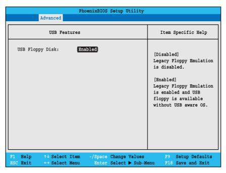
Figure 11. USB Features Submenu
